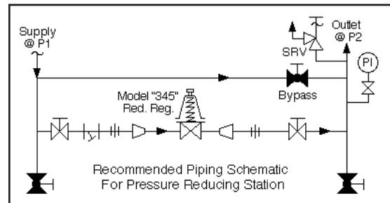
8. Flow Direction: Install so the flow direction matches the arrow cast on the main regulator body.
