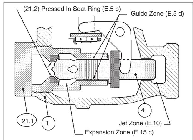
**Cylinder Sub-Assembly (21) with Piston (24) Metal Seat Construction**
