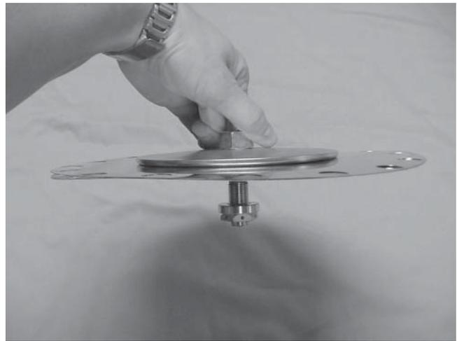
Diaphragm sub-assembly consists of items (10), (11), (12), (13), (15), (16) and (20). (Metal diaphragm design).
