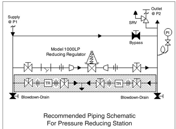
6. Clean the piping of all foreign material including chips, welding scale, oil, grease and dirt before installing the regulator. Strainers are recommended.
